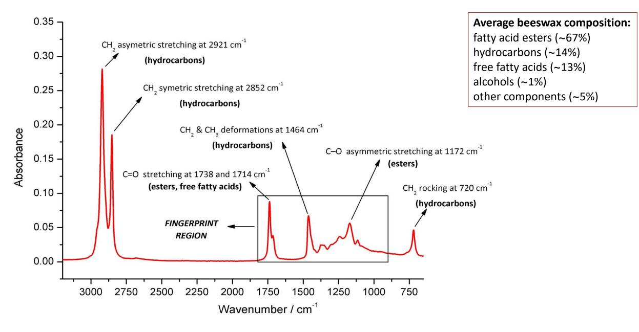
Characteristic FTIR-ATR spectrum of *A. mellifera* beeswax with assignation of underlying molecular vibrations (absorption bands)
