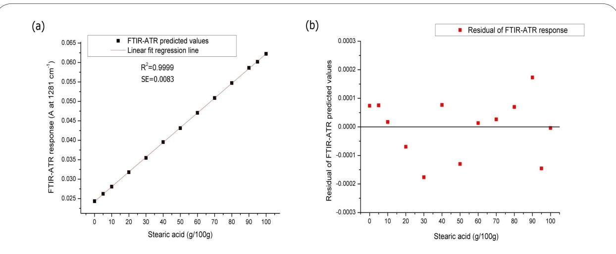
(a) Prediction performance parameters of the calibration curve constructed for determination of the stearic acid share in beeswax: a scatter plot of instrument response data (FTIR-ATR predicted values) vs. real stearic acid share values;
